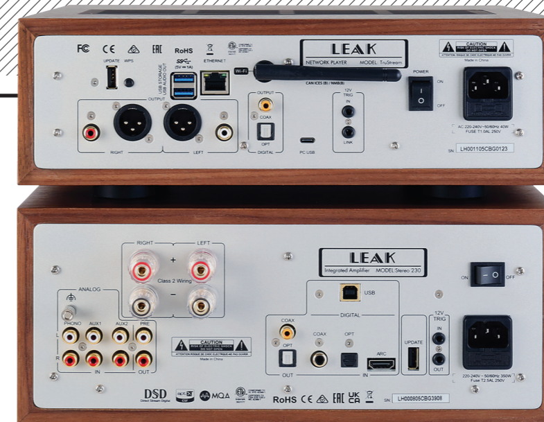
ABOVE: The TruStream [top] offers Wi-Fi/wired Ethernet and USB-C inputs (to 768kHz/DSD512), two USB host ports, coax/opt digital outs and RCA/balanced XLR analogue outs. The Stereo 230 [bottom] also has coax/opt in/out, an HDMI ARC in, plus three line and one MM phono input. Speaker outs are on 4mm binding posts
