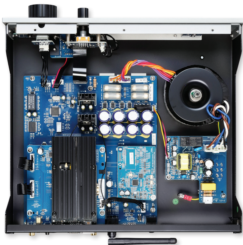
ABOVE: Linear PSU [top right, and standby below] feeds XMOS USB board [bottom centre] and Silent Angel-based wireless/Ethernet/USB streaming platform [under heatsink], with ES9038Q2M DAC-based preamp [below]
